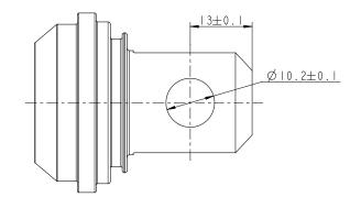
Option "2" and "B" LINAK P/N: 0251010 with bushings, Zinc coated steel 0251014 with bushings, Stainless steel AISI 304
