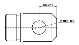
Option "2" and "B" Piston 0231016 with bushings, Zinc coated steel Piston 0231095 with bushings, Stainless steel AISI 304
