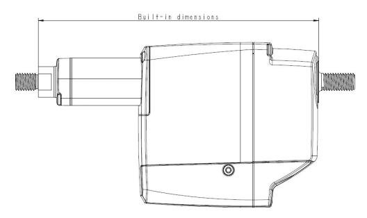
The built-in dimensions for options M and F are measured according to this illustration.
