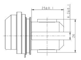
Option "3" and "C" LINAK P/N: 0251010 without bushings, Zinc coated steel 0251014 without bushings, Stainless steel AISI 304
