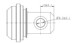
Option "5" and "F" LINAK P/N: 0251032 without bushings, Zinc coated steel 0251034 without bushings, Stainless steel AISI 304
