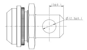
Option "8" and "1" LINAK P/N 0251032 with bushings, Zinc coated steel 0251034 with bushings, Stainless steel AISI 304
