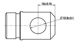
Option "4" and "D" Piston 0231033 with bushings, Zinc coated steel Piston 0231096 with bushings, Stainless steel AISI 304
