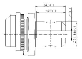
Option "6" and "G" LINAK P/N: 0251026 with bushings, Zinc coated steel 0251033 with bushings, Stainless steel AISI 304
